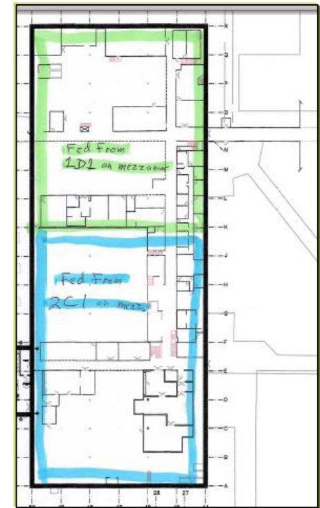
Map building to substations
